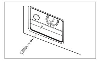
4 Unscrew the screw from the lower side of the cabinet cover.
