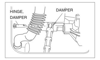
1 Disassemble the damper hinges from the tub and base.
