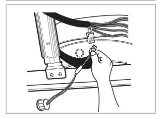
4) Disassemble the lamp assembly.
