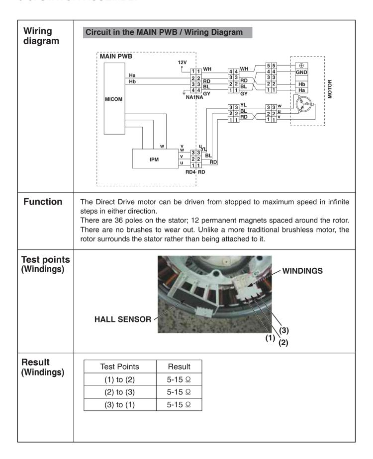
The hall sensor determines the speed and direction of the motor. It also can read that the load is off balance when the drum speed fluctuates.
