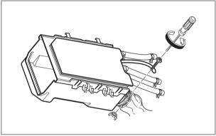
4 Unscrew the clamp nut at the lower part of the dispenser.
