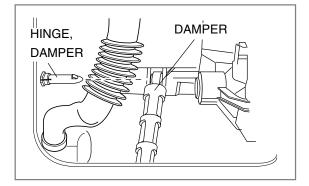
① Disassemble the damper hinges from the tub and base.
