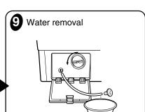
· If SERVICE is needed during check, remove the remaining water by pulling out the hose cap.
