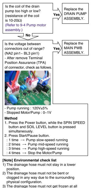
4) The drainage pump must not have any improper
