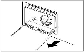
③ Put a flat ( - ) screwdriver or putty knife into the hinge slots at the bottom of the cover and pry it out.
