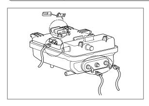
Remove the housing attached to the TSG. (Heater, Water level frequency-sensor, Thermistor.)
