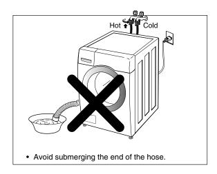
$\divideontimes$  The end of the drain hose should be placed less than 96" from the floor.
