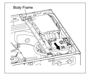
(5) Remove the body frame and then separate the TSG from the washer.
