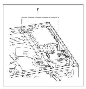
(3) Remove the screws from both ends of the frame rail.
