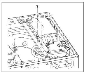
② Remove the screw of the TSG and body frame.
