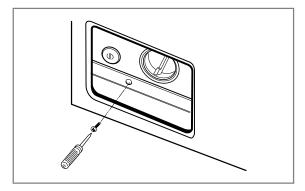
4 Unscrew the screw from the lower side of the cabinet cover.
