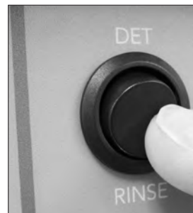
Push DOWN and HOLD until you see air bubbles moving through the rinse-aid tubing.
