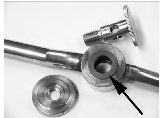
Clean the upper and lower rinse arm bearings.
