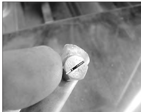
Clean the final rinse arm nozzles.
