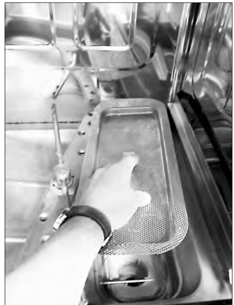
Remove the scrap screen
